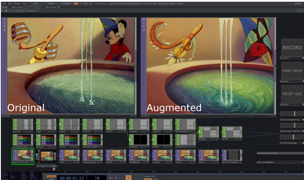
Figure A.2: Screenshot of the Generative AI Pipeline implemented inside TouchDesigner . The EEG-derived control value is used to steer the image-to-image diffusion model, which augments the frames of a movie in real-time.
